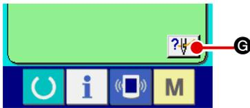
④ **Display the threading diagram.**
